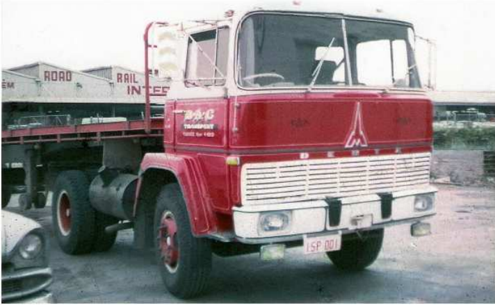
Pluto V8 tilt cab model from 1968. The split windscreen was an Australian modification
