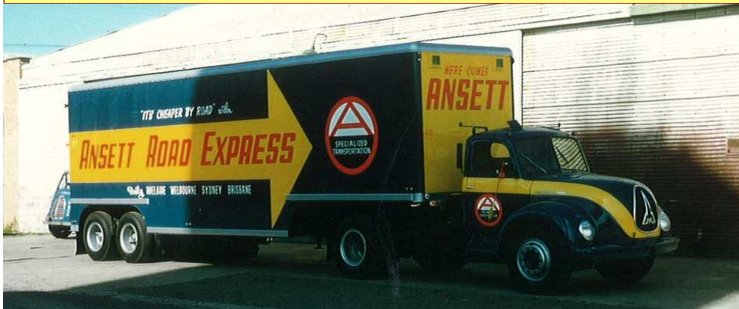
An Ansett Jupiter and "Cargo Clipper" c 1956. The bogie trailer was built largely of aluminium and Firestone air suspension was used on some units.
